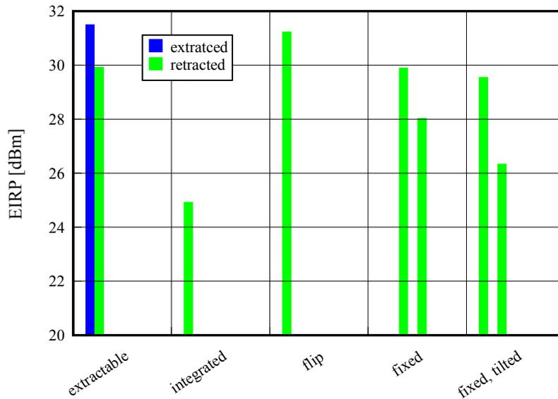
Fig. 4: Measured GSM 900 EIRP values for different mobile phones as a function of the implemented antenna concept.
