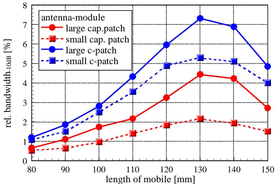
Fig. 4: Relation between impedance bandwidth and length of the mobile (simulation).
