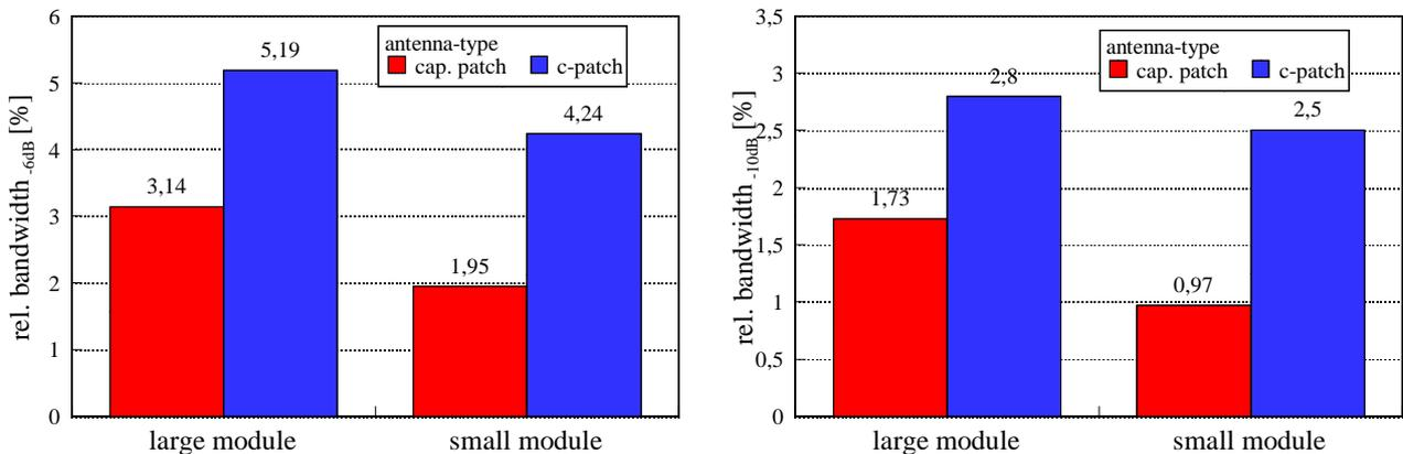
Fig. 3: Relative impedance bandwidths (925 MHz) of capacitively loaded patch and c-patch (simulation).
