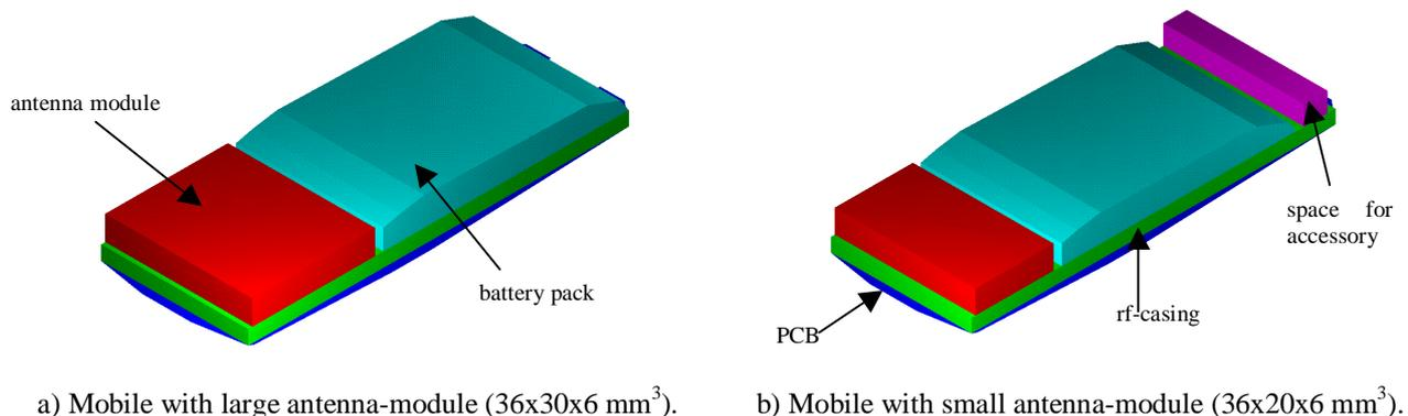
Fig. 2: Mobile with two different restrictions to the antenna volume.
