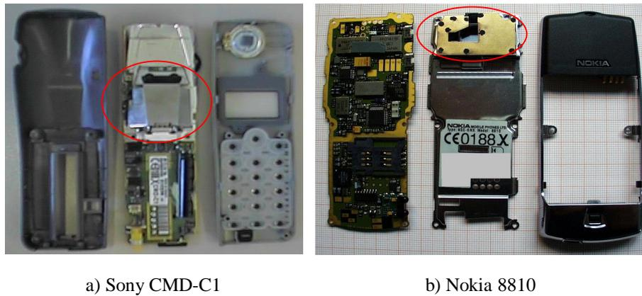
Fig. 1: Mobile phones with integrated antennas.
