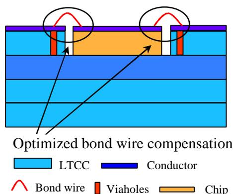
Figure 1: Side view of the microstrip / coplanar chip feed.
