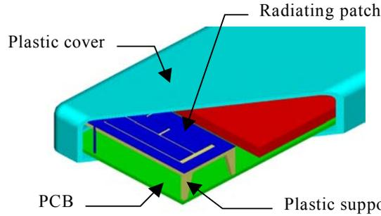
Fig. 1: Integrated patch antenna with a plastic carrier.
