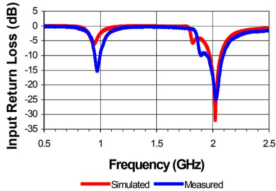
Fig. 2: Simulated and measured input return loss of the triple-band antenna
