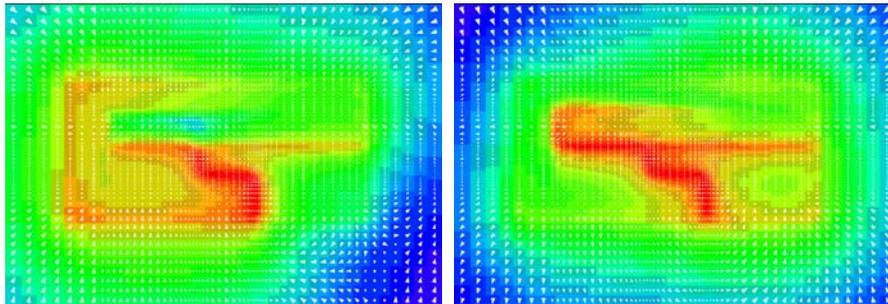
Fig. 5: Electric nearfield of the antenna normalized to its maximum,  $f=900$  MHz. Antenna without support (left), and with a 1 mm-thick plastic carrier,  $\epsilon_r=4.5$  (right).
