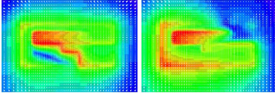
Fig. 6: Electric nearfield of the antenna normalized to its maximum,  $f=2$  GHz. Antenna without support (left), and with a 1 mm-thick plastic carrier,  $\epsilon_r=4.5$  (right).
