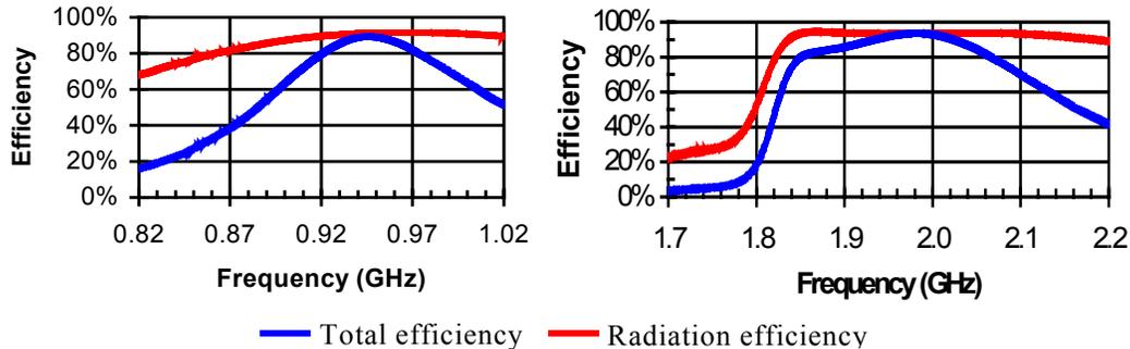
Fig. 3: Antenna efficiency for the GSM (left) and DCS/PCS (right) frequency bands
