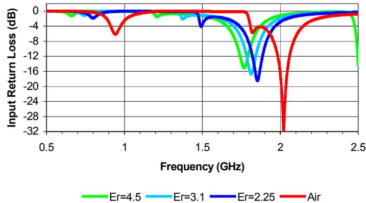
Fig. 4: Input return loss with different plastic carriers, made of different, commercial plastics.
