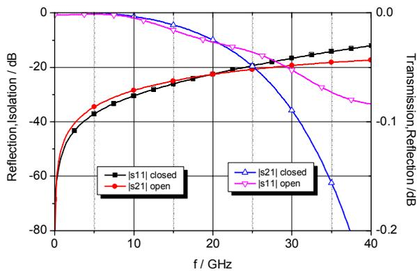
Fig. 6: Simulation results of the Toggle-Switch in open and closed position.
