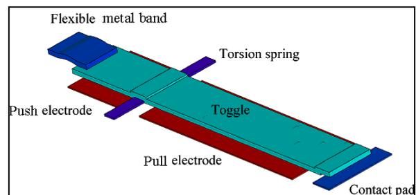
Fig. 1: Schematic view on the Toggle switch
