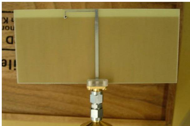
Fig. 17: Measurement setup with antenna on FR-4
