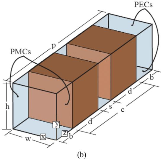
Fig. 1: 1D CDP PPWG structure. The propagation direction is  $z$ . (a) Perspective view. (b) Unit cell (PECs on top and bottom sides perpendicularly to  $y$ , PMCs on left and right sides perpendicularly to  $x$ ).
