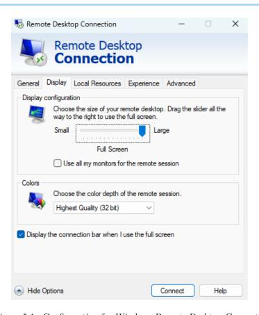
Figure 5.1.: Configuration for Windows Remote Desktop Connection
