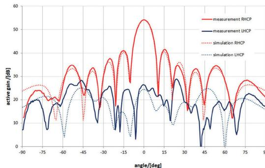
Antenna Farfield pattern simulation vs. measurement
