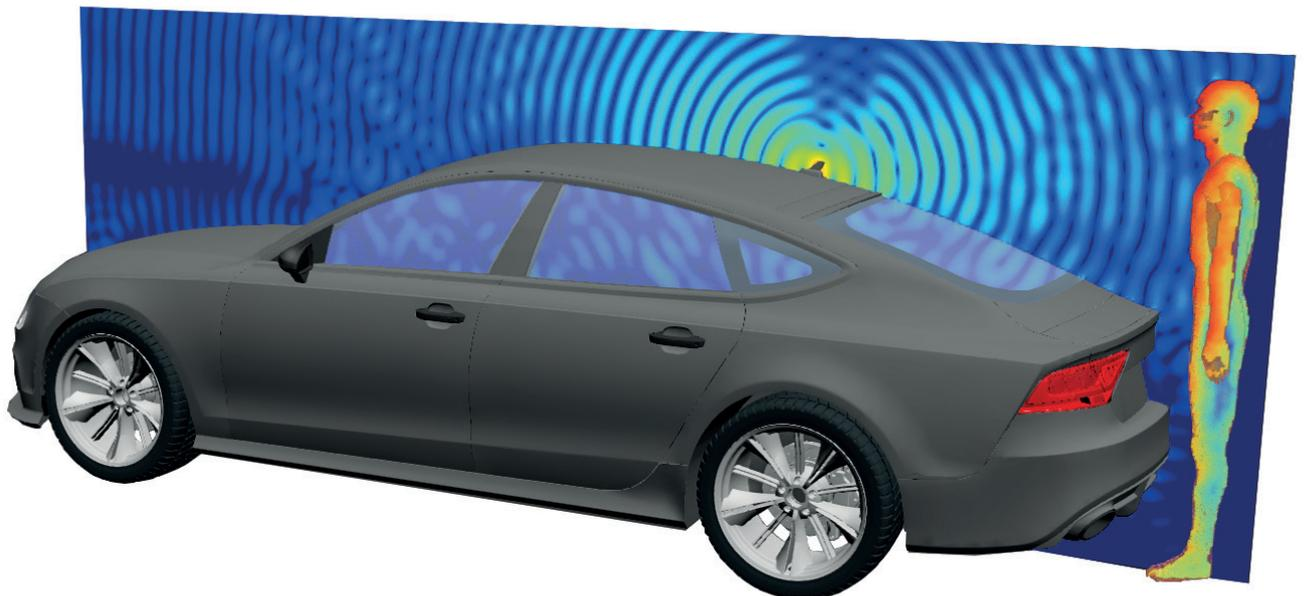
3D EMPIRE model of vehicle with bystander showing electric field and specific absorption rate (SAR) in body model
